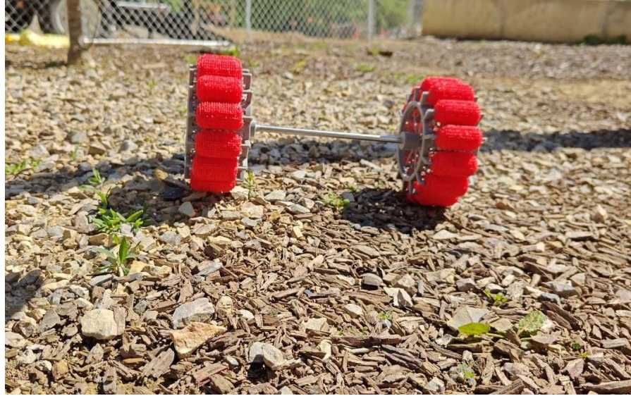
Figure 19: Dust shedding test over a non-homogeneous surface consisting of organic matter, dust, and stones of varying sizes
