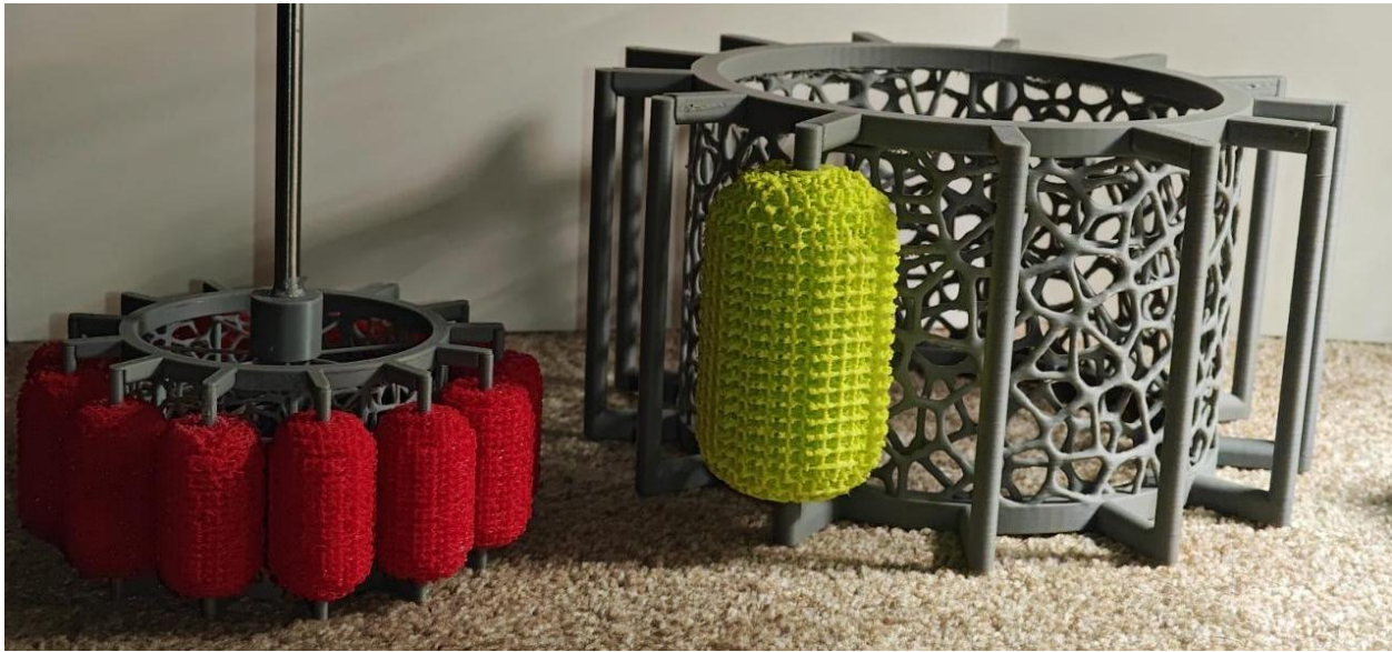
Figure 21: Left: 1:2 Scale prototype wheel system (Grey = PLA; Red = TPU); Right: 1:1 Scale prototype wheel system (Grey = PLA; Neon Yellow = TPU)
