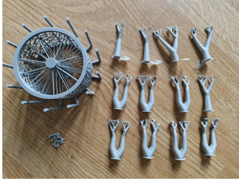
Figure 18: PLA parts printed in grey color, depicting the Ti components (the structures on right are the organic tree support structures used for printing the main component)
