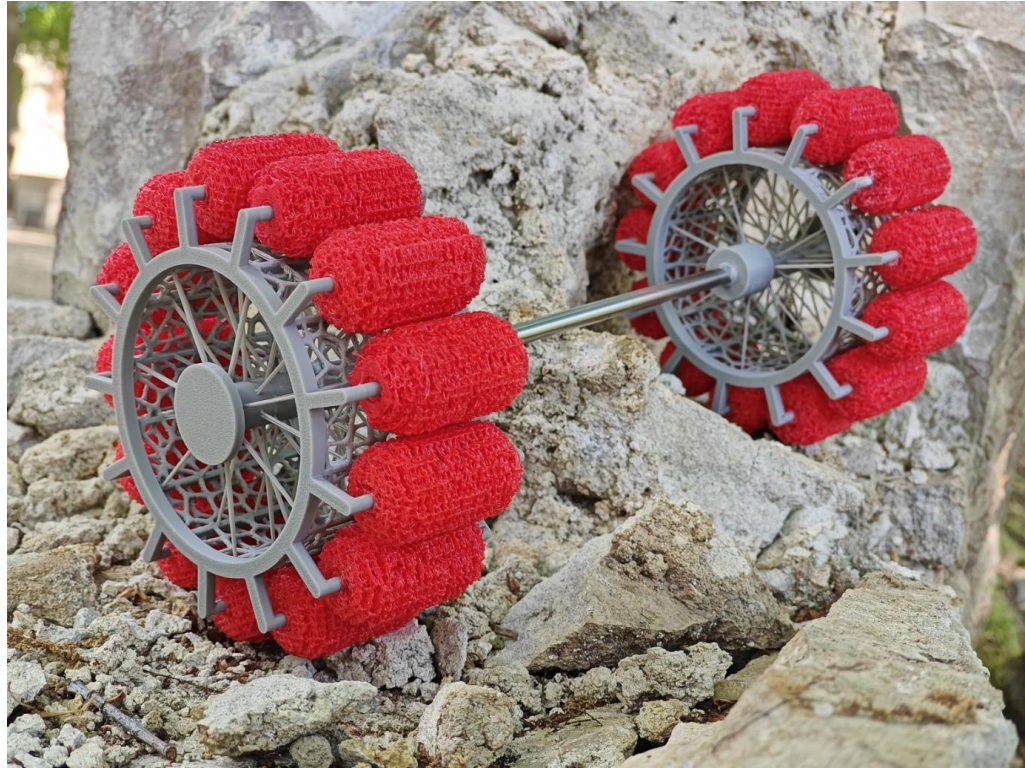
Figure 20: Prototype wheel being tested on broken concrete slabs and structures. Modular TPU lugs offered consistent grip across slope gradients and irregular textures, supporting the intended use case of Martian surface mobility where regolith, rock fragments, and slopes interact unpredictably.
